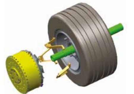
Conceptual view of the Smart Operation on Ground motor attached to the A320 wheel
