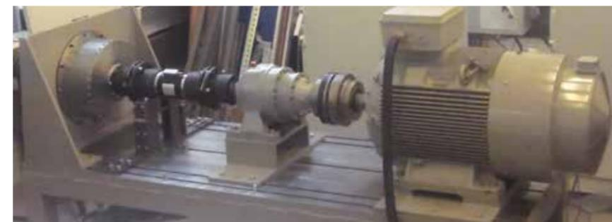
The Smart Operation on Ground motor test-rig in the University of Nottingham laboratories (SOG motor is on the far left)
