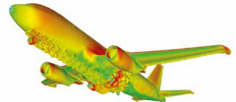
RANS-LES CFD simulation obtained for Nose Landing Gear in Take-Off condition of  $\alpha=10.5$ , 180kt, sea level  $M=0.272$  (Courtesy FOI)
